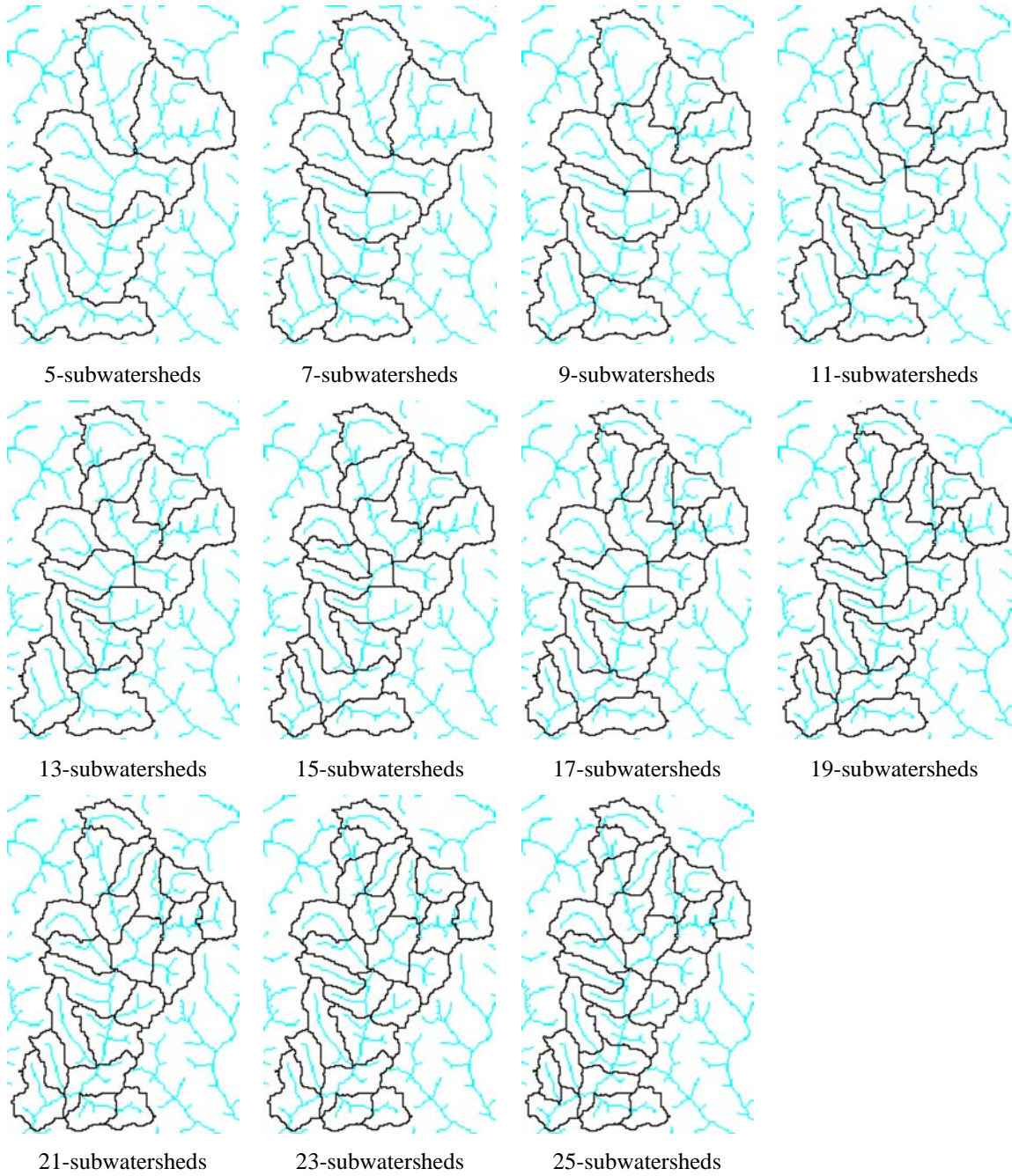
Figure 7.5: Orientation of sub-watersheds in cases used to study effect of watershed subdivision
