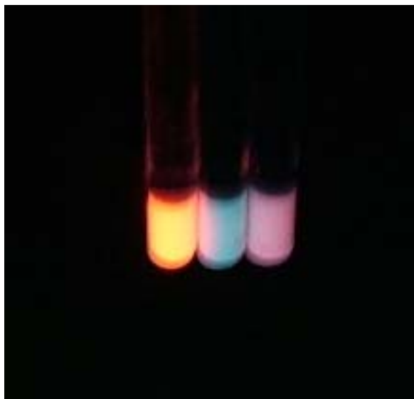
Figure 5.60. Photograph of Eu:BioMOF-1, Tb:BioMOF-1, and Sm:BioMOF-1 (from left to right) under D 2 O, illuminated by an Entela Mineralight lamp (model UVGL-55) with 365 nm excitation (115 V, 0.16 amp); a 450 nm glass cut-on filter was placed in front of the camera lens to remove the UV light.
