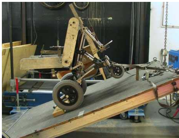
Figure 23: Static stability test of PALM v2
