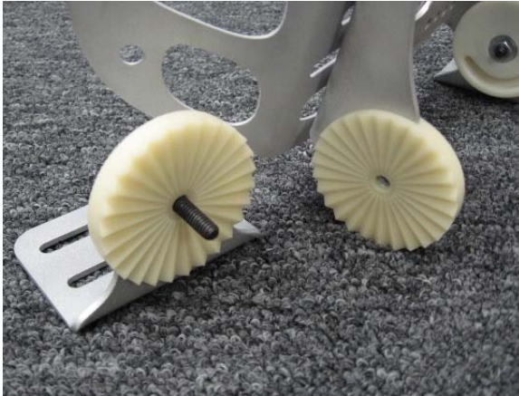
Figure 40: Close-up of adjustment mechanism used at back rest recline and leg rest angle points.
