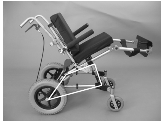
Figure 17: Side view of U.S. PALM. Improvements to linkage geometry were made between versions.
