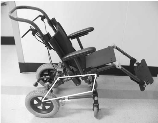
Figure 16: Side view of India PALM in tilted position. Lines indicate position of four bars in linkage.
