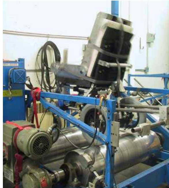
Figure 24: US PALM on double drum test machine
