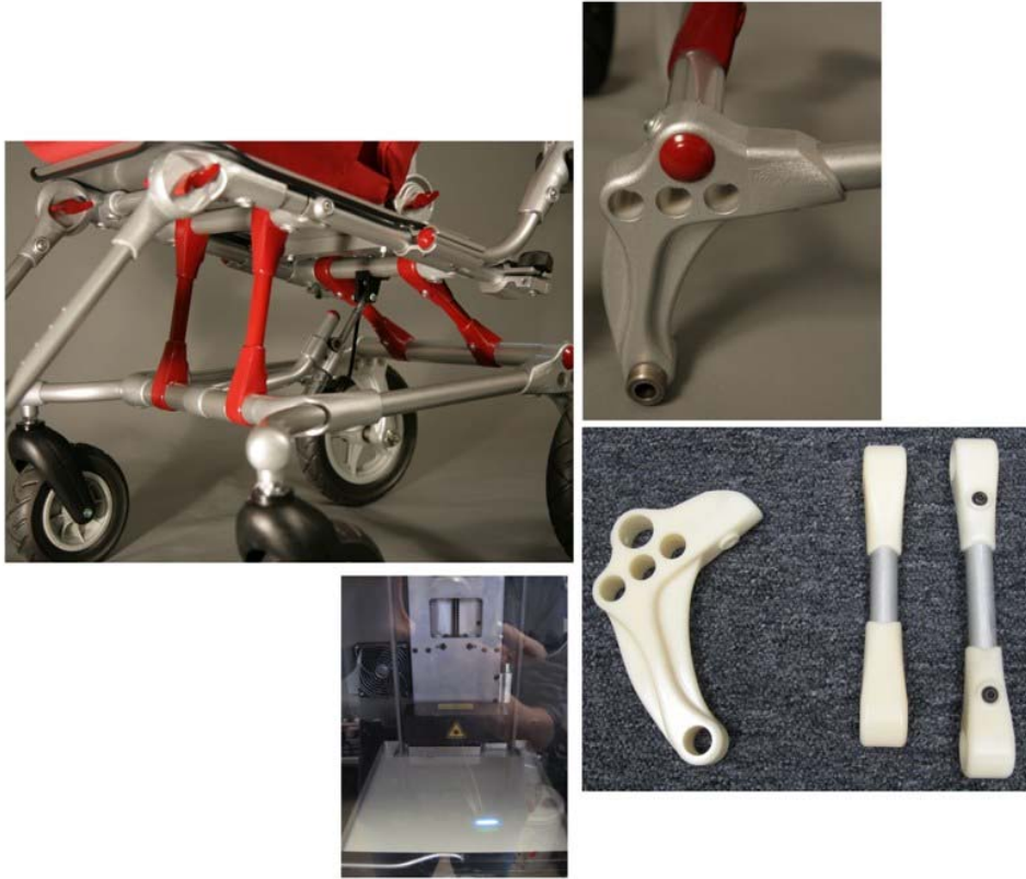
Figure 12: Images of SLA process. Vat in which parts are made, Unpainted SLA parts and SLA parts finished and assembled on final prototype
