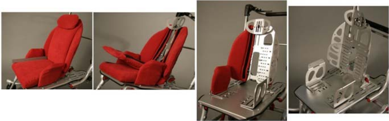
Figure 32: Upholstery adheres to seat frame with Velcro, is removable and washable.
