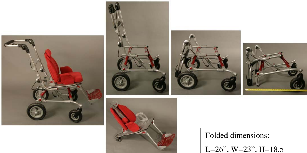
Figure 28: Process of dismantling Final PALM for transport
