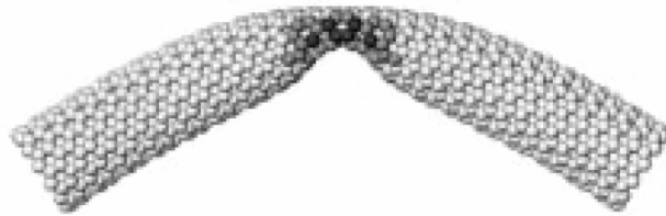
Figure 5. Simulated bending of a nanotube under a deforming force. Deformation is elastic rather than permanent. Reproduced with permission from B.I. Yakobson et al., Phys. Rev. Lett. 1996, 76, 2511 [32]. Copyright 1996, American Physical Society.
