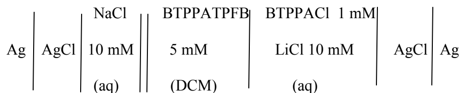
Figure 9.1 Representation of the blank electrochemical cell employed in all measurements
