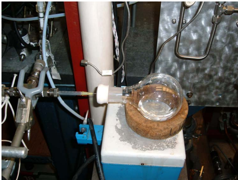
Figure 6.1 Setup of Headspace Collection using a 250 mL RB flask and sealed with a septum. Notice the modified hypodermic syringe.
