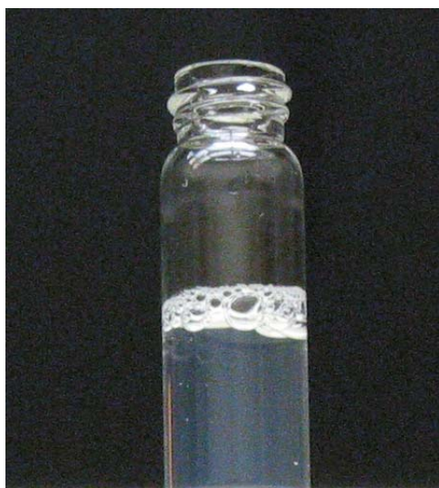
Figure 11. Transparent NIPAM solution at 25 °C. Swollen particles, ~ 200 nm diameter.
