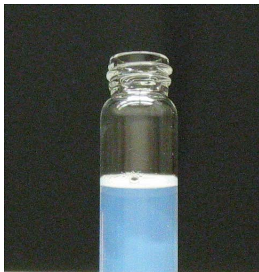
Figure 12. Turbid NIPAM solution at 45 °C. Collapsed particles, ~ 50 nm diameter.
