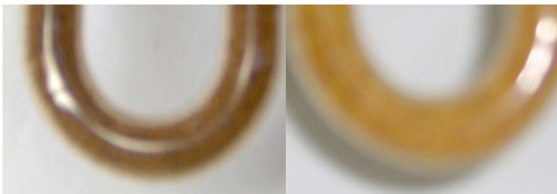
Figure 20. Color of chromium oxide catalyst depending on dominant state of oxidation. A: +3, B: +6
