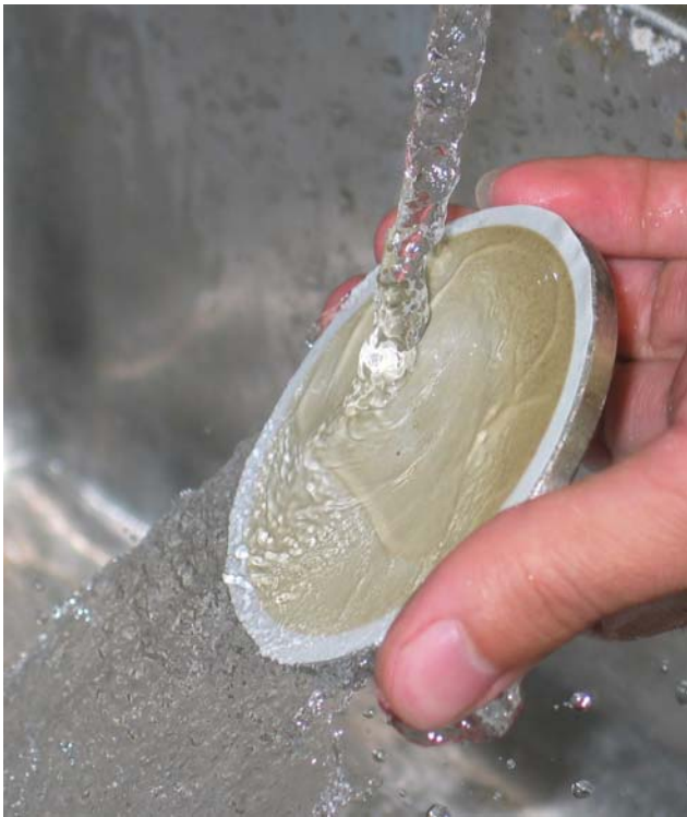
(b) Hotter (53 °C) tap water flushing at a flow rate about 3.6 \text{ m}^3/\text{m}^2 \cdot \text{s}
