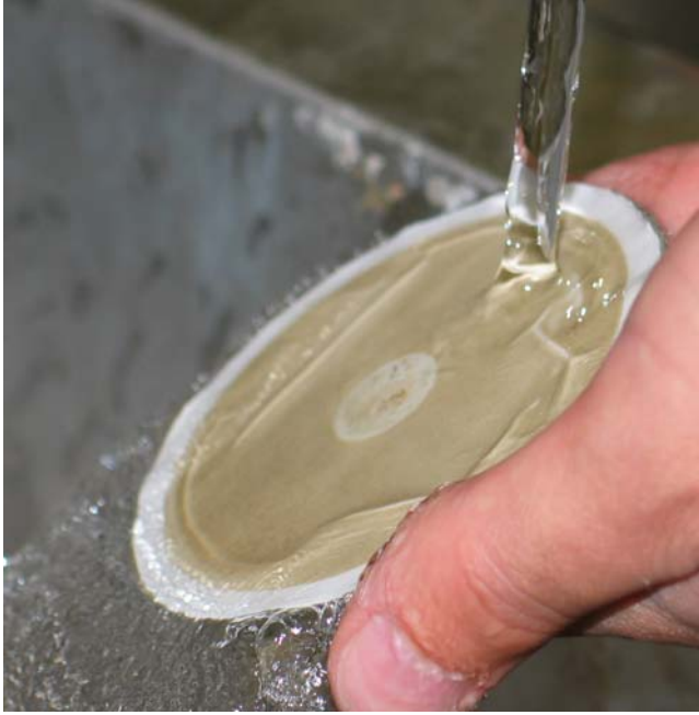
(a) Warm (38 °C) tap water flushing at a flow rate about 1.9 \text{ m}^3/\text{m}^2 \cdot \text{s}
