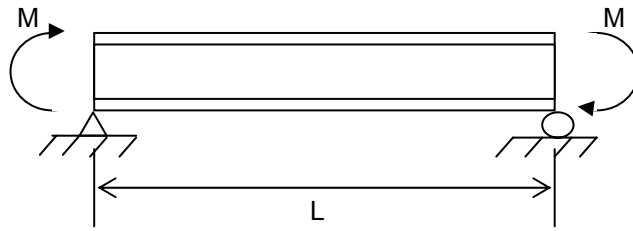
Figure 10.37 Simple Beam with Equal and Opposite End Moments
