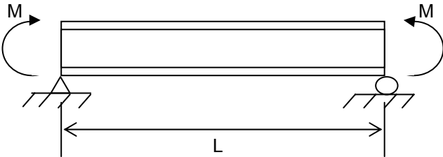
Figure 10.32 Simple Beam with Equal End Moments
