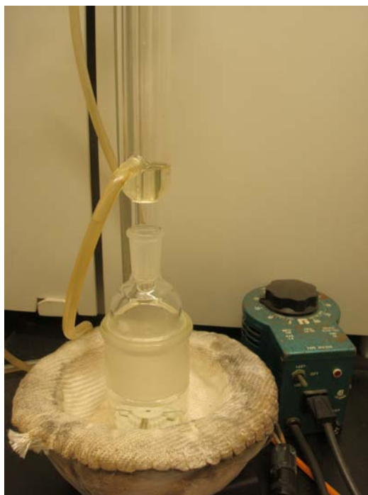
Figure A-3. Photograph of the flat-bottom flask connecting with the Liebig condenser sitting in a heater with sand.
