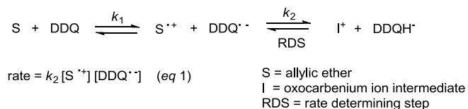
Figure 11. Reaction rate analysis
