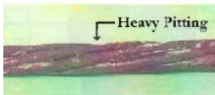
(e) corroded strand with heavy pitting.
