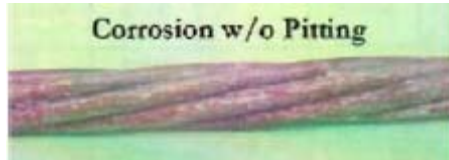
(c) corrosion without pitting (strand intentionally cut).
