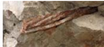
(c) corrosion without pitting (strand intentionally cut).
