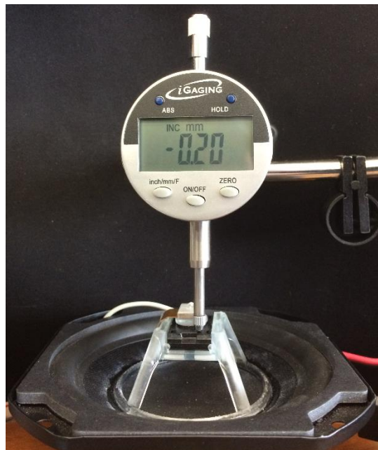
Figure 8. Apparatus for calibration of displacement using mechanical gage, shown with a current in the voice coil causing the speaker cone to be displaced downward by 0.20 mm.
