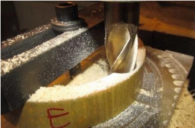
(a) End mill cutting of modified test specimens in operation ( \beta = 0 , \alpha = 0.20 and \gamma = 0.80 shown)
