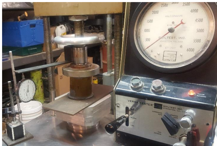
(b) Image of compression test set-up.
