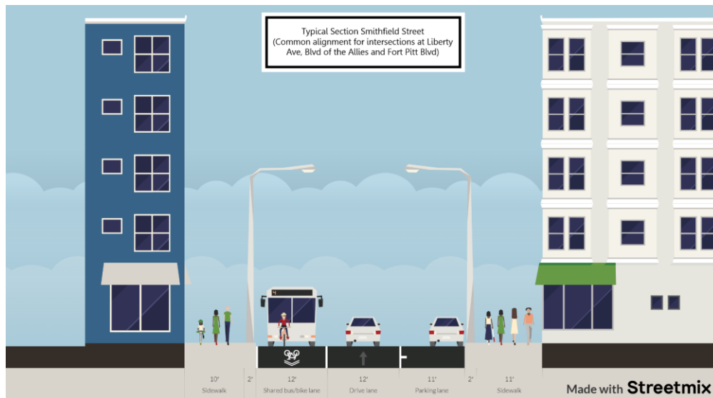
Figure 28: Typical section for majority of Smithfield Street
