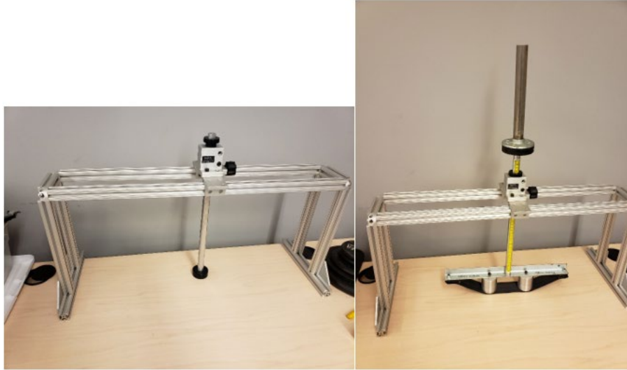
Figure 8. The Apparatus of Loaded Contour Depth and Overload Deflection
