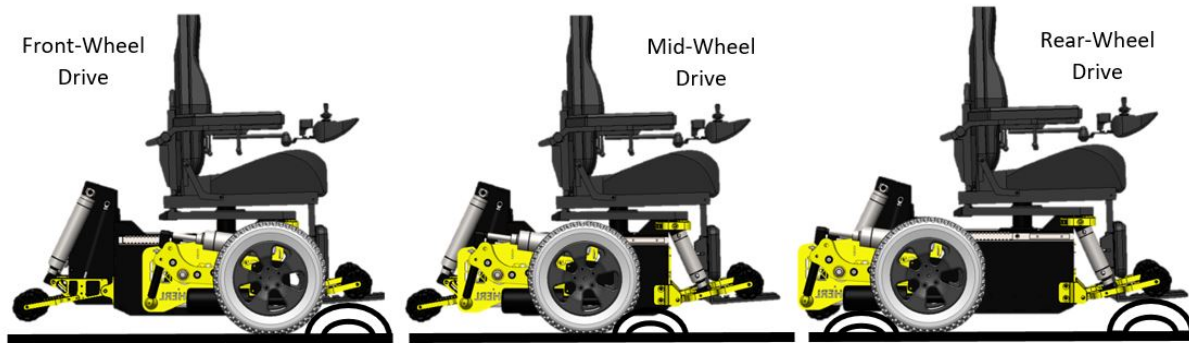
Figure 1: MEBot 's drive wheel configuration upon obstacles
