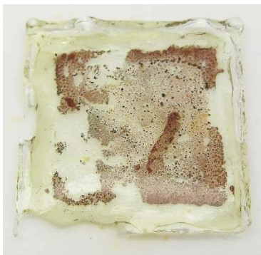
Figure 3.8 A \text{Cu}^{2+} -doped hydrogel, after electrochemical reduction for 30 hours at -0.2 V in 0.1\text{M KNO}_3/0.1 M urea aqueous electrolyte shows over-reduction to \text{Cu}^0 , likely due to the presence of Cu ions in the electrolyte.
