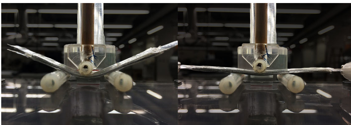
Figure 5.17 Tri-layer PEAA-TMA sample at 12% RH under an applied load of 2.5 N at 0 V (left) and 450 V (right) applied potential.
