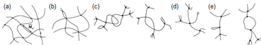
Figure 1.4 Representation of network structure in hydrogels. (a) ideal network. (b) Multifunctional crosslinks. (c) Physical entanglements. (d) Unreacted dangling ends. (e) Loops.
