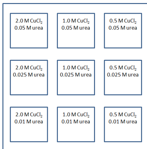
Figure B.2 A diagram of nine samples doping with different concentrations of copper and urea to determine the optimum concentration for future doping experiments.
