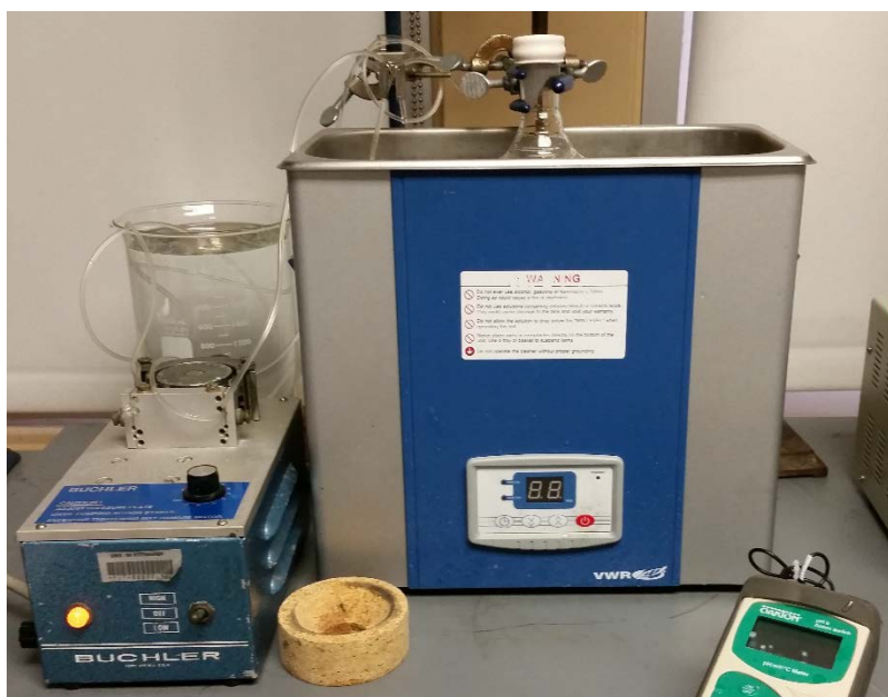
Figure 13. Experimental Set-up for Graphene Synthesis. 500-mL round-bottom flask reaction vessel suspended in VWR Ultrasonic Cleaner (Model #97043-988). Buchler peristaltic pump and 2000-mL water reservoir used to maintain level of water bath. Also shown Oakton pH6 Acorn Series pH/mV/°C meter used to monitor sonication bath temperature.
