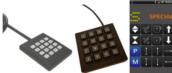
Figure 3. The iARM 16 keys of the Medium & Large keypad are provided with numbers and letters (0-9 and A-F) and the user interface of the Android application (iMove).
