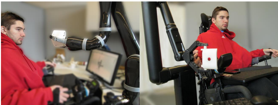
Figure 2. Two commercialized wheelchair-mounted robotic manipulators: JACO manipulator (left) and Manus ARM (right).
