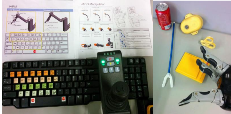
Figure 7. Left: ARM user interfaces and instructions; Right: The daily objects that can be used for the WMFT-ARM – soda can, mouth stick, lock or keyhole, key, and pad
