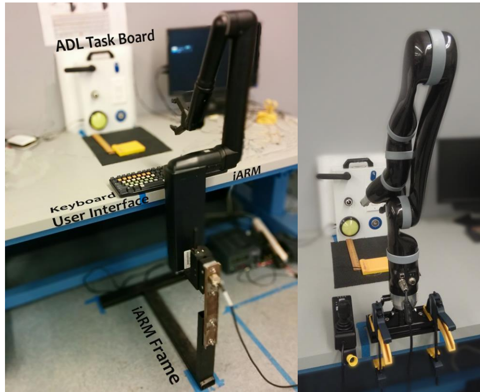
Figure 11. Subject testing set up for the iARM and JACO ARM
