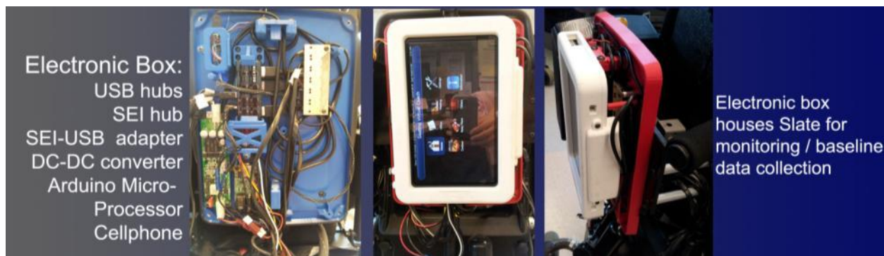
Figure 3. The electronic box of the tablet VSC. [1]
