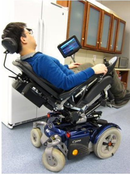
Figure 1. The sensors are installed on the wheelchair for the tablet virtual seating coach. [1]
