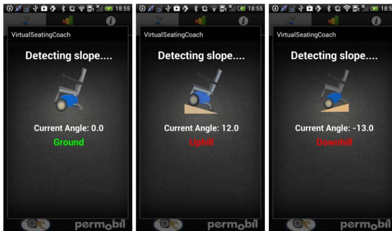
Figure 24. When the slope detection function is initialized, it will detect if the wheelchair is on a slope and display the information on the screen.
