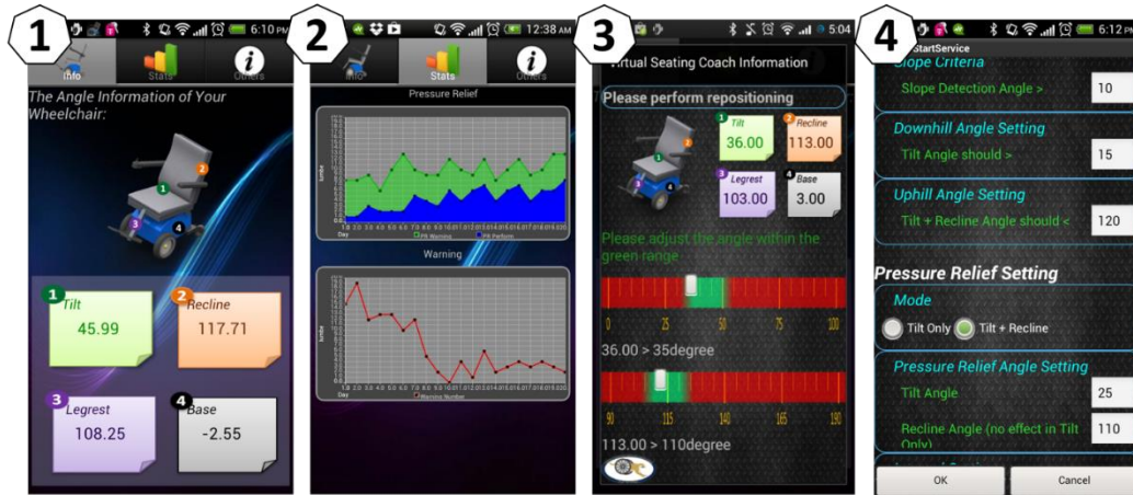
Figure 18. Screenshots of the Smartphone Virtual Seating Coach application. (1) Main Menu : Showing the angles of the powered wheelchair, including seat tilt, backrest recline, legrests elevation and wheelchair base inclination. (2) Statistics display of powered seating functions usage : Users can review their progress of using seating functions. The goal is to increase the compliance with performing repositioning and decrease the number of seating function usage warnings. (3) Instruction Menu : Instructing the users to adjust their wheelchair. The angle bars highlight the target angles in green based on the clinical recommendations. The white indicators point out the current seating angles and move as the user adjusts the seating angles. (4) Clinician Setting : Clinicians can customize reminder and warning parameters for users.
