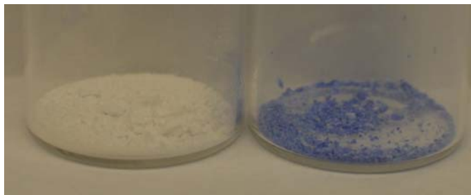
Figure 5.26. Picture comparing the colors of Yb(BTC)(H 2 O) nanoMOF ( left , white) and Yb(BTC)(H 2 O)+4hAQ ( right , blue).
