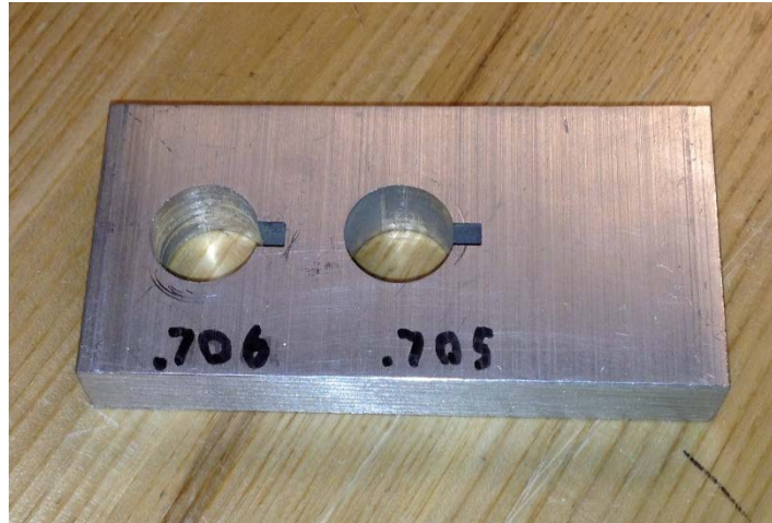
Figure 31. Hub motor axle test component
