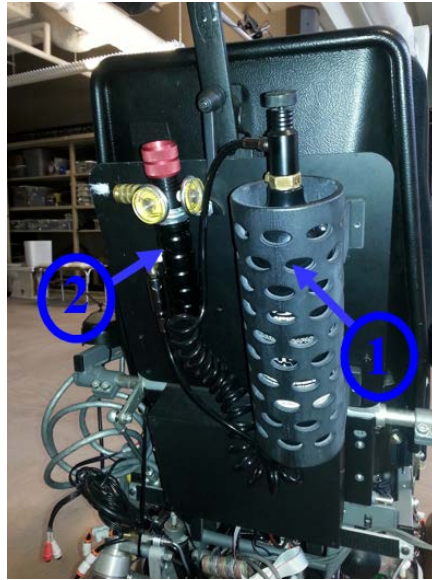
Figure 11. CO2 tank (1) and expansion chamber (2)
