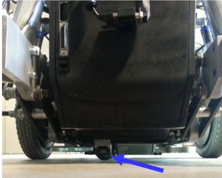
Figure 10. Driving wheel electric actuator clearance in lowest position
