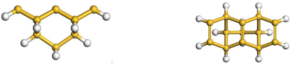
Figure 19: The three dimer Si 13 H 12 surface model cut from the optimized p(2x1) flat surface. The side view is on the left and the top view is on the right.
