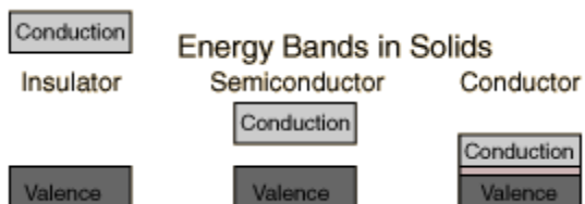
Figure 8: Semiconductors have band gap with widths between those of insulators and metals.
