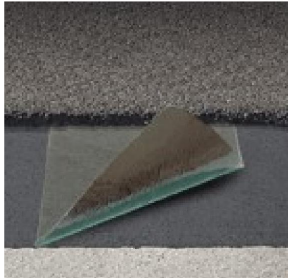
Figure 4.7: Polymer modified asphalt waterproofing membrane with adhesive
