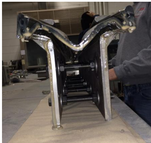
Figure 3.11: Strip seal joint fixture used in experiment
