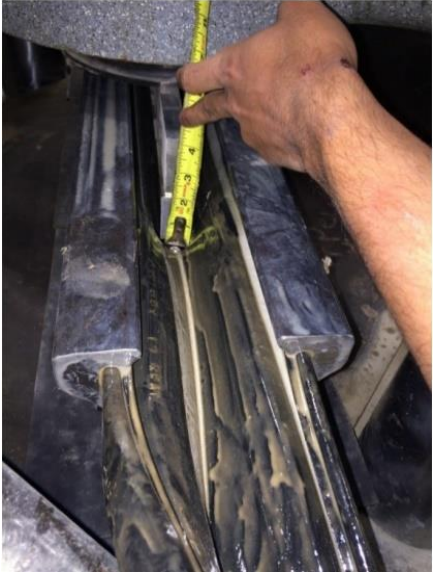
Figure 3.13: Around 4 in. deflection at the end of loading
