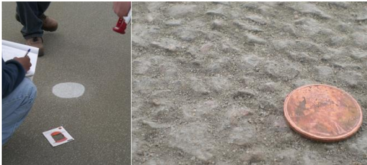
Figure 3.9: Sand Patch Test for Evaluating EAC Texture and EAC Texture Closeup
