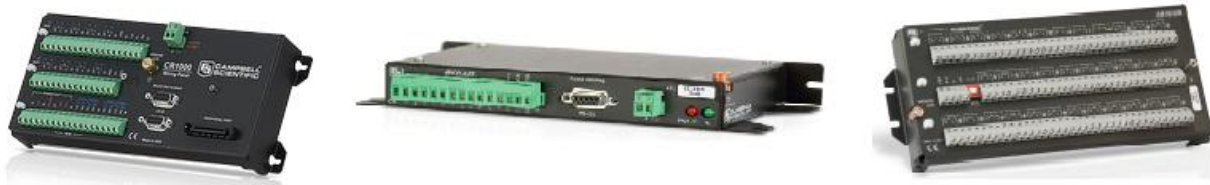
Figure 3.17: Datalogger and Peripherals Needed for Collecting Data from MnROAD Sensors [28]
