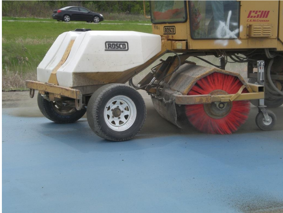
Figure 3.8: Tractor Mounted Brush Attachment for Providing EAC Finish
