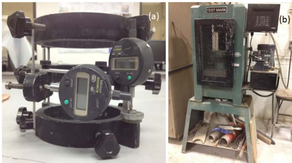
Figure 3-4. Apparatus for compressive strength test and Young's Modulus & Poisson's Ratio measurement: (a) Concrete Elastic Modulus Meter, (b) TEST MARK CM4000 compression machine
