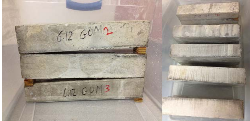
Figure 3-9. Thawing phase setup
