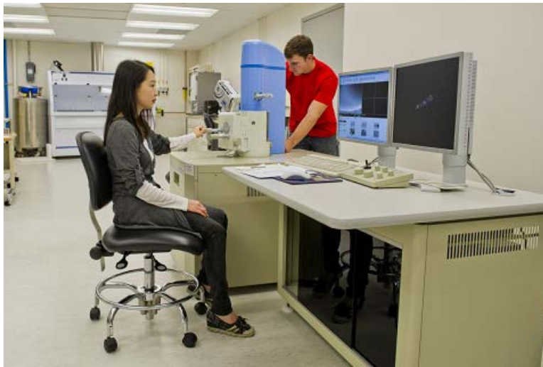
Figure 5-14. JEOL JSM-6510LV/LGS scanning electron microscope (PINSE, 2014)
