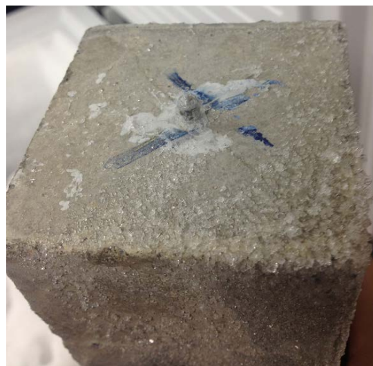
Figure 3-6. Stainless steel rods embedded in the end
