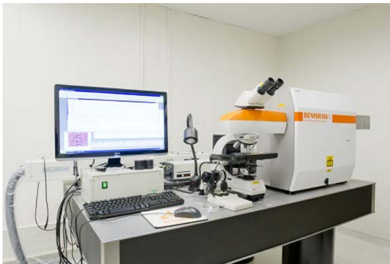
Figure 5-9. Renishaw inVia Raman microscope (PINSE, 2014)
