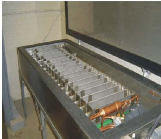
Figure 2-4. Freezing and thawing machine (Hamoush et al. 2012)
