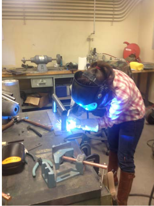
Figure 13. Grab Bar being welded to Securement Plate
