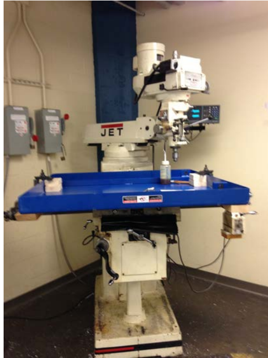
Figure 7. Scissor Lift Table Top being Manually Milled
