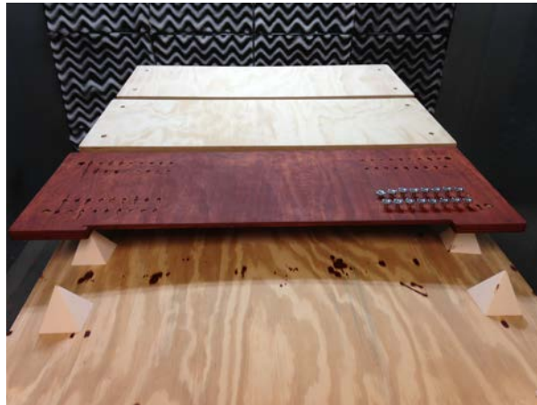
Figure 6. Transfer Platform Board Being Stained
