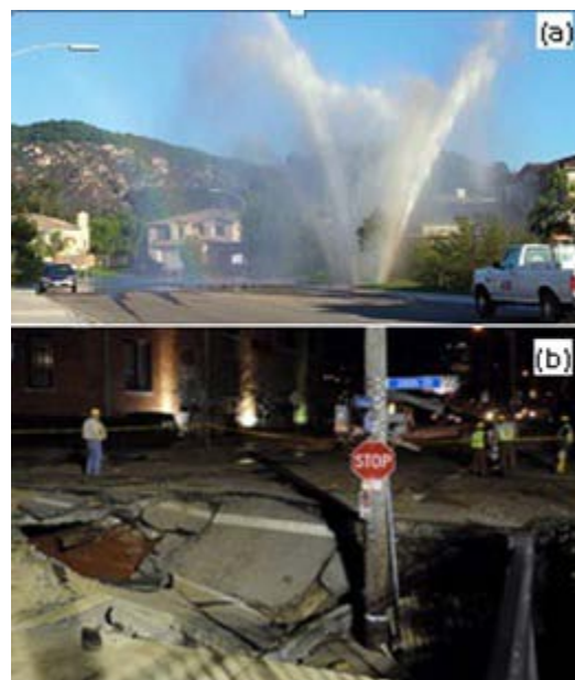
Figure 1.1. (a) Picturesque photo of a water main break [2]. (b) Street collapse due to a water main break [3].
