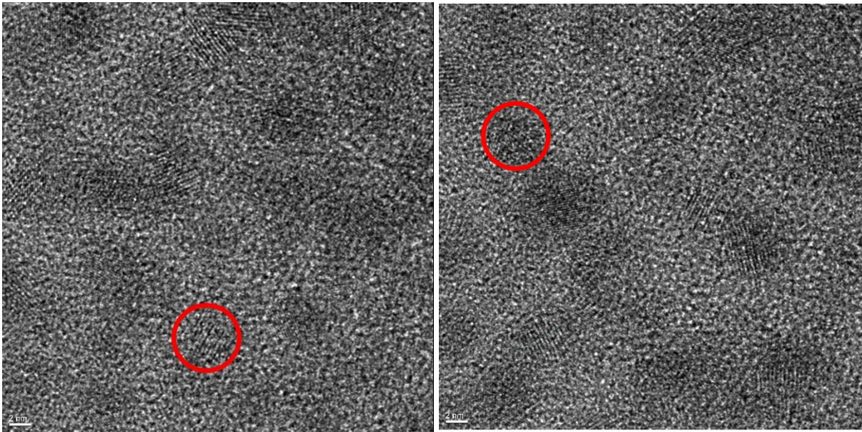
Figure 11: TEM images of CdSe:Tb particles. The scale bars are 2 nm. Crystal structure is easily observed in these images, verifying that nanocrystals are present.
