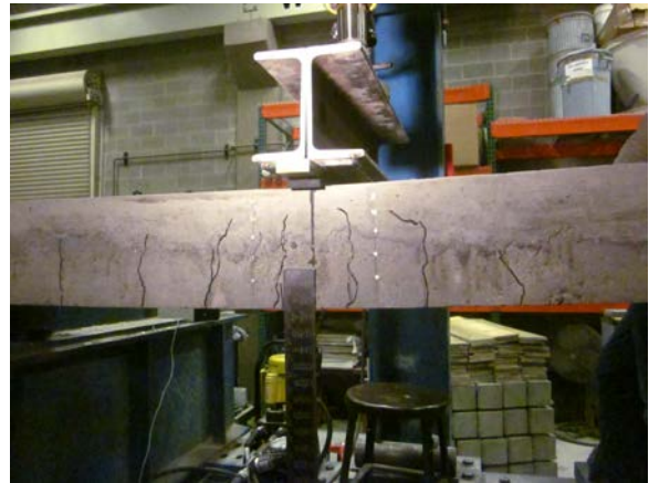
e) Final DEMEC Reading (49.3 kipft)
