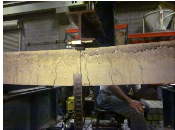
e) Final DEMEC Reading (66.7 kipft)
