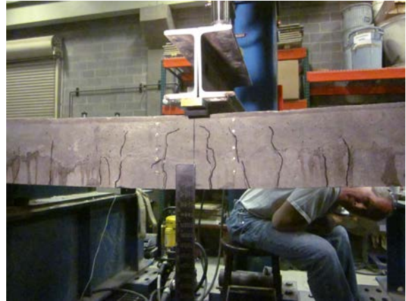
e) Final DEMEC Reading (45.7 kipft)
