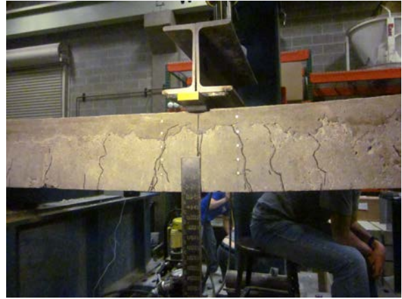
e) Final DEMEC Reading (56.3 kipft)
