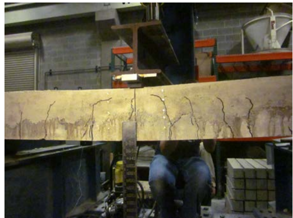
e) Final DEMEC Reading (47.5 kipft)
