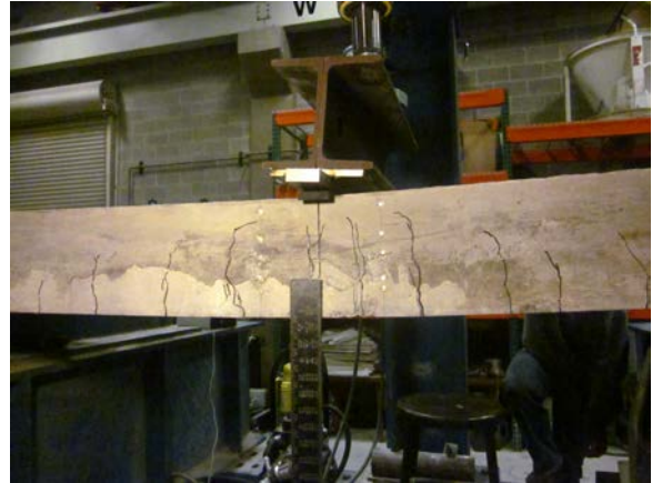
e) Final DEMEC Reading (49.1 kipft)
