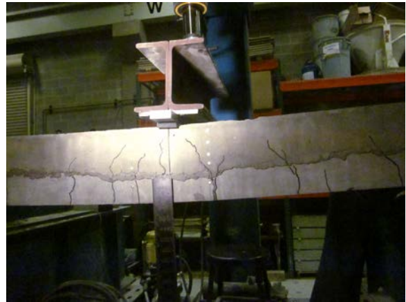
e) Final DEMEC Reading (42.3 kipft)
