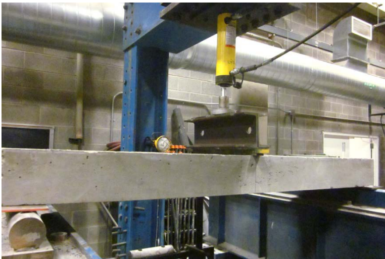
a) Test Set-up (Slab A shown)
