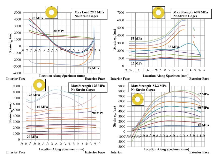
Figure A-1: Specimen TG1-1 (Free): Inner (Upper Left), Middle (Upper Right), Outer (Lower Left), & Radial (Lower Right)
