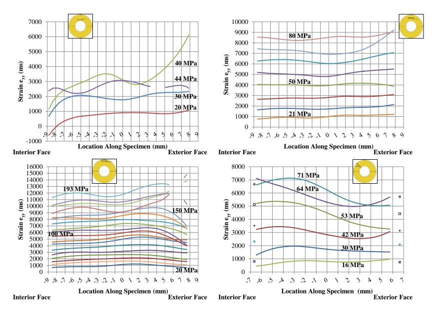
Figure A-21: Specimen TG21-13 (Free): Inner (Upper Left), Middle (Upper Right), Outer (Lower Left), & Radial Manual Values (Lower Right)
