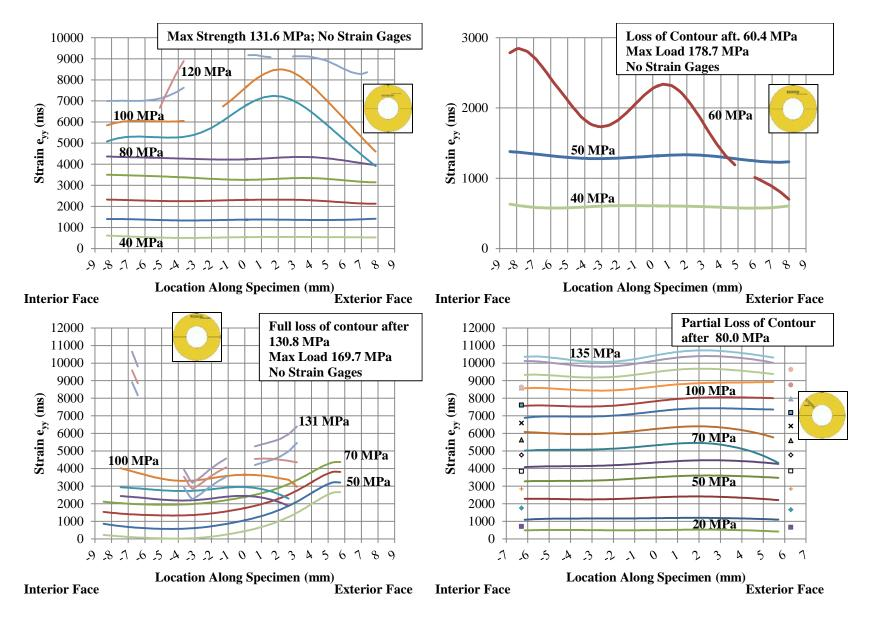
Figure A-6: Specimen TG1-6 (Fixed): Inner (Upper Left), Middle (Upper Right), Outer (Lower Left), & Radial (Lower Right)
