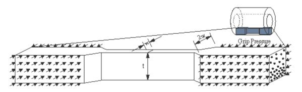
Figure 3-1: Representative bamboo dogbone specimen
