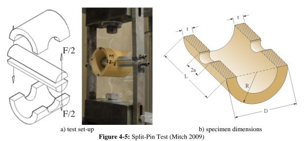
Sharma (2010) sought to develop a less complex test that could be applied in the field and correlate with the split-pin test which requires specimen machining, a complex test apparatus and a method of applying tension; all impractical in a field test. The edge bearing test, shown in Figure 4-6, was proposed as a surrogate for the more complex split-pin test, since a compression
