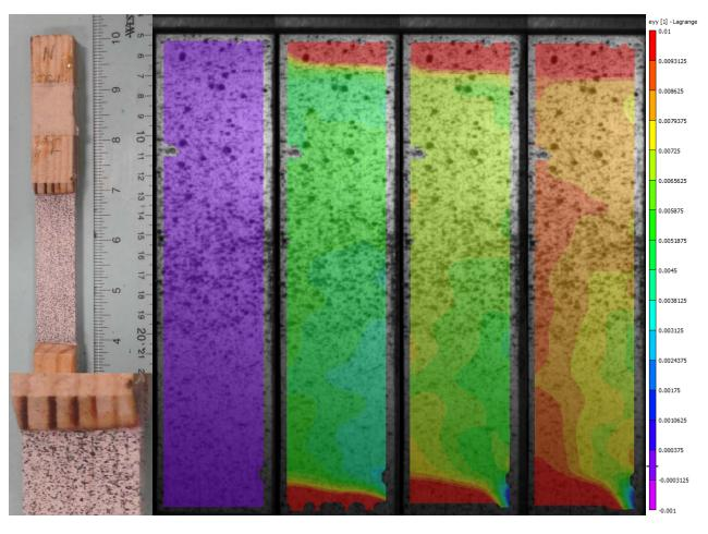
Figure A-44: Contour Banding in Radial Free Specimen TG21-12
