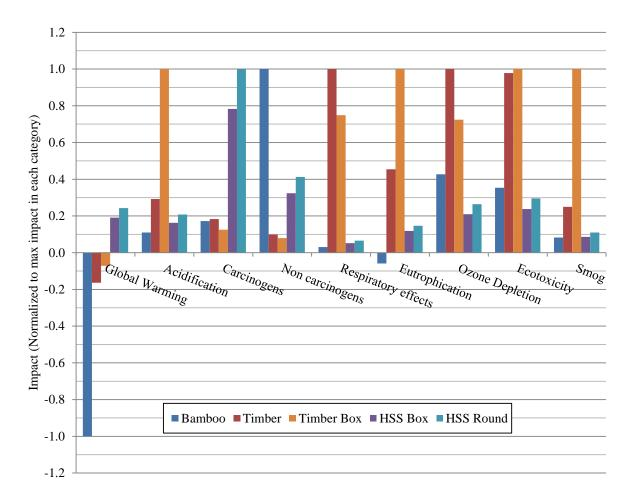
Figure 6-5: LCIA profiles for bamboo, timber, and steel columns (scenario 2)
