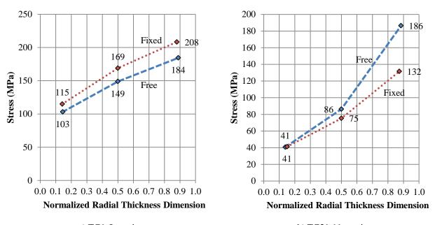
a) TG1-5 specimens b) TG21-11 specimens **Figure 3-18:** Representative stress profiles for specimens TG1-5 and TG21-11
