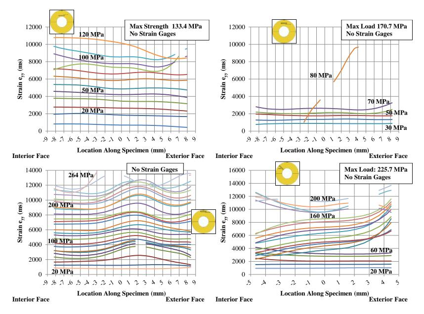
Figure A-11: Specimen TG1-9 (Free): Inner (Upper Left), Middle (Upper Right), Outer (Lower Left), & Radial (Lower Right)
