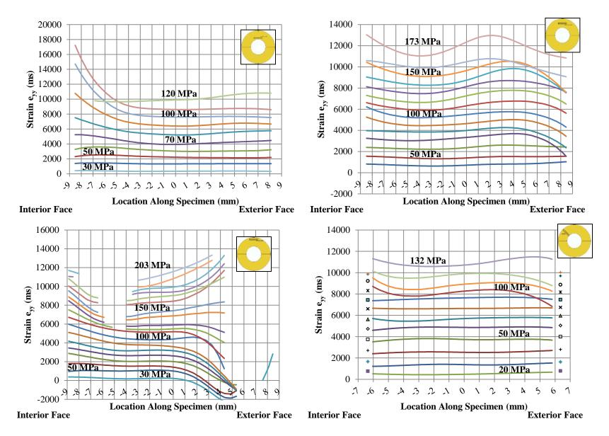
Figure A-5: Specimen TG1-6 (Free): Inner (Upper Left), Middle (Upper Right), Outer (Lower Left), & Radial (Lower Right)
