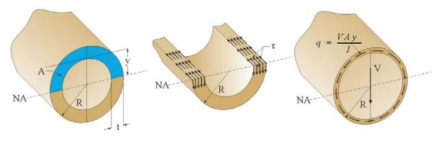
(a) Shear in thick-walled tube
