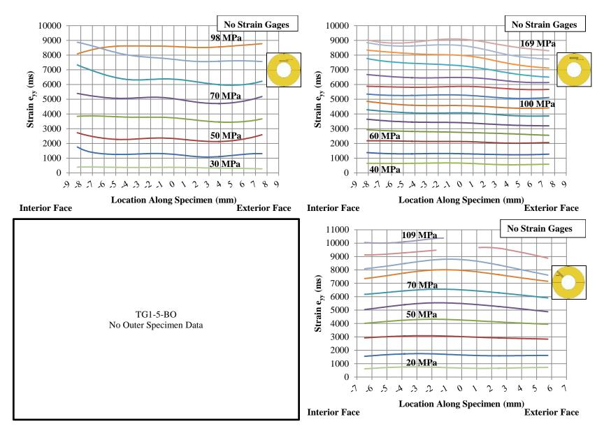
Figure A-4: Specimen TG1-5 (Fixed): Inner (Upper Left), Middle (Upper Right), Outer (Lower Left), & Radial (Lower Right)
