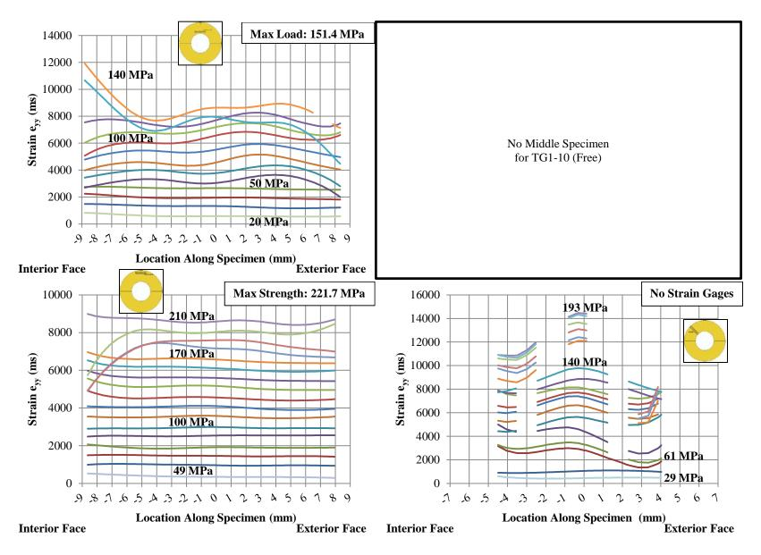
Figure A-13: Specimen TG1-10 (Free): Inner (Upper Left), Middle (Upper Right), Outer (Lower Left), & Radial (Lower Right)
