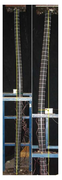
Figure 5-3: Buckled shaped of PVC columns 1 and 2
