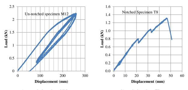
a) un-notched specimen M12 b) notched specimen T8 Figure 4-15: Representative load-displacement curves
