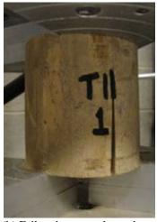
(a) Failure at shear plane(b) Failure between shear planesFigure 4-7: Examples of Bowtie Test Failure Planes
