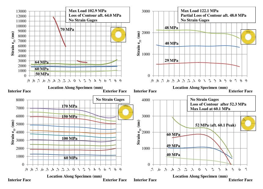
Figure A-10: Specimen TG1-8 (Fixed): Inner (Upper Left), Middle (Upper Right), Outer (Lower Left), & Radial (Lower Right)
