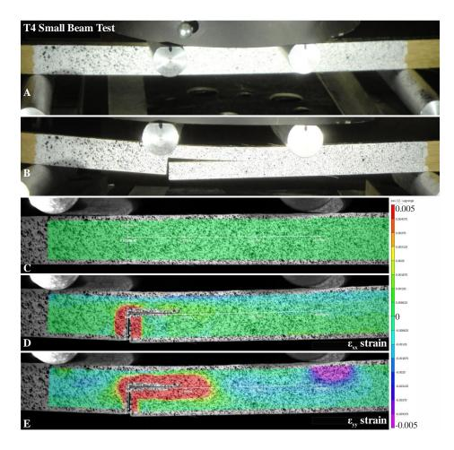
Figure 4-11: VIC-3D Contour Images for Notched Tre Gai Specimen
