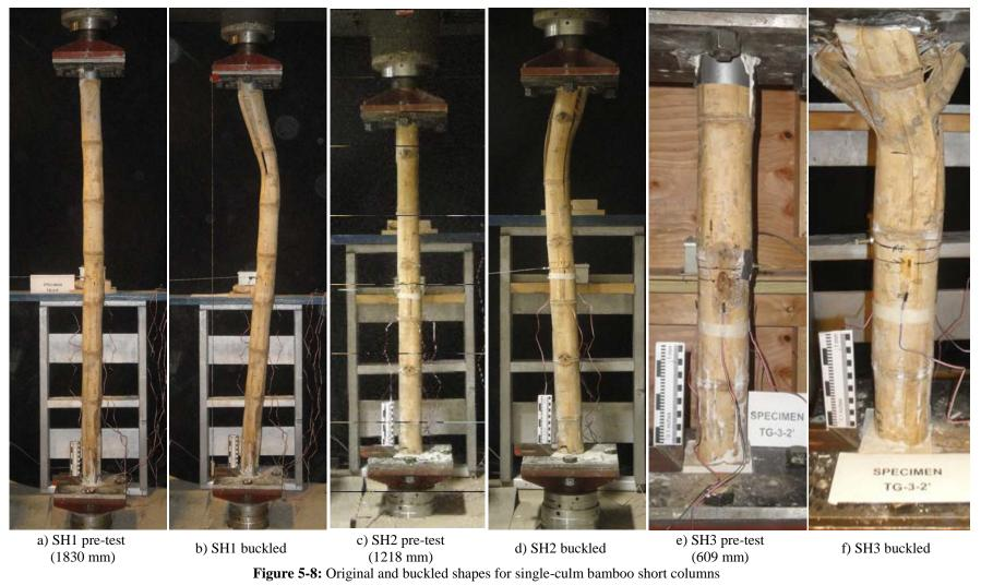
The results of the short column tests indicate some additional limitations of such tests and emphasize the sensitivity of bamboo material and member tests to support or boundary conditions. Such sensitivity, one assumes, is carried into real structures and must be addressed in design standards – most likely through reduced material reduction factors.
