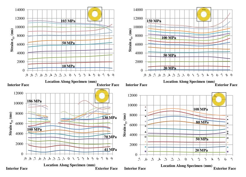
Figure A-3: Specimen TG1-5 (Free): Inner (Upper Left), Middle (Upper Right), Outer (Lower Left), & Radial (Lower Right)
