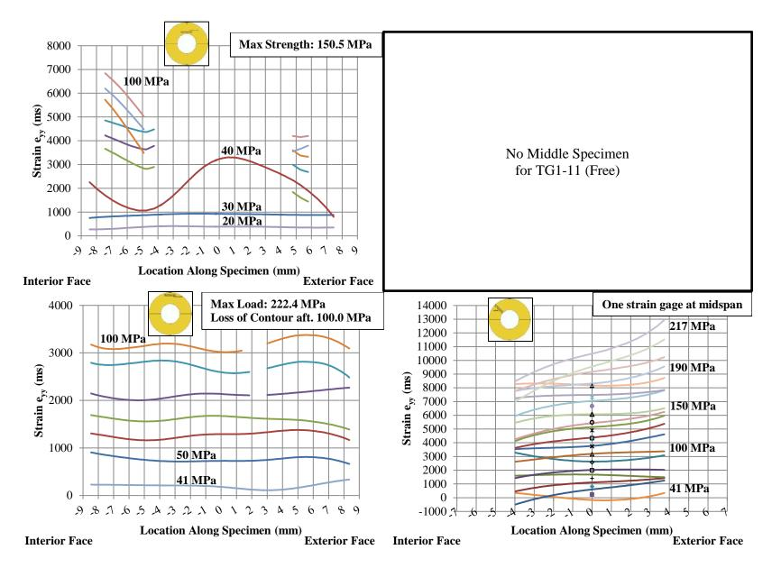
Figure A-15: Specimen TG1-11 (Free): Inner (Upper Left), Middle (Upper Right), Outer (Lower Left), & Radial (Lower Right)
