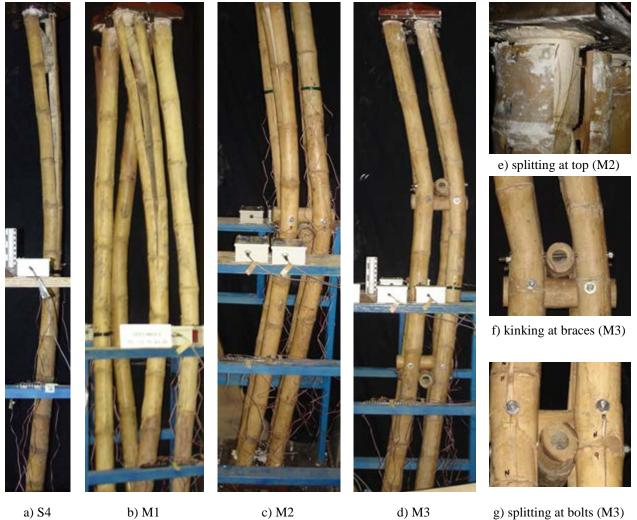
b) M1 c) M2 d) M3 Figure 5-6: observed behavior of bamboo column specimens
