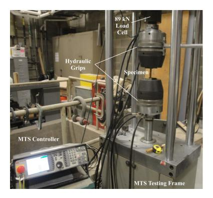
Figure 3-8: Experimental Test Set Up
