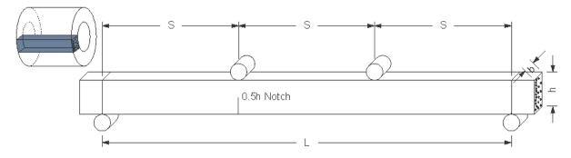
a) test set-up orientation and dimensions
