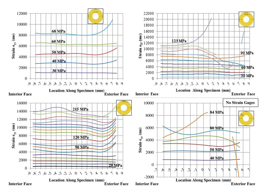
Figure A-20: Specimen TG21-12 (Fixed): Inner (Upper Left), Middle (Upper Right), Outer (Lower Left), & Radial (Lower Right)
