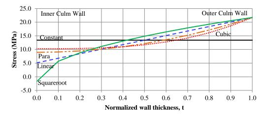
Figure 3-5: Stress due to uniform strain
