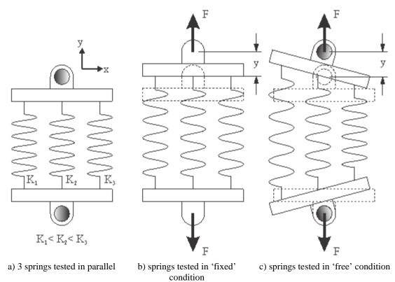
Figure 3-3: Rotation in representative spring model loaded in Tension
