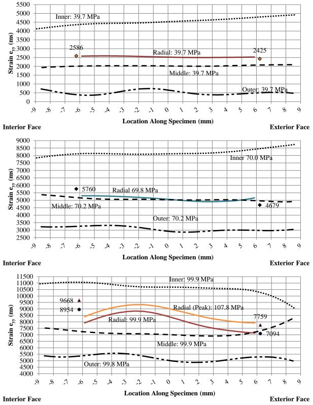
Figure 3-16: Strain profile for specimen TG1-5 (free): 40MPa (top), 70 MPa (center), and 100MPa (bot.)
