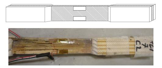
Figure 3-10: Location of strain gages on tension specimen and gages after testing
