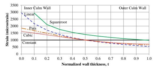
Figure 3-6: Total strain including rotation of moment Fe
