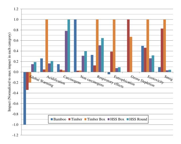
Figure 6-4: LCIA profile for bamboo, timber, and steel columns (scenario 1)
