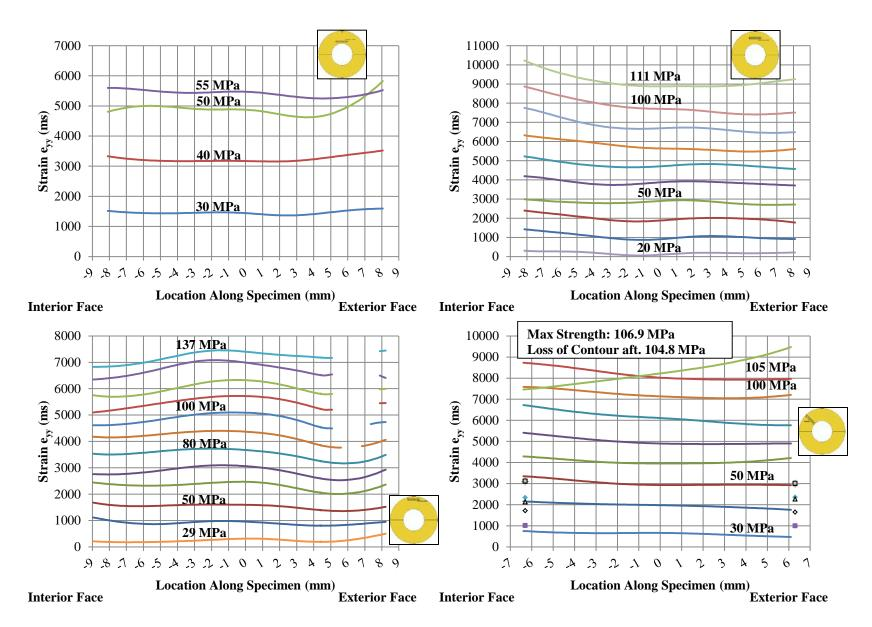
Figure A-19: Specimen TG21-12 (Free): Inner (Upper Left), Middle (Upper Right), Outer (Lower Left), & Radial (Lower Right)
