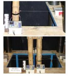
d) DWT instrumentation at midheight of single culm (top) and fourculm (bottom) test. Figure 5-4: Test set-up and instrumentation
