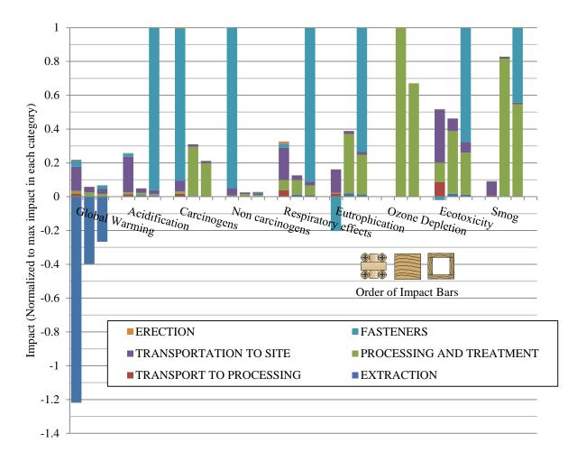
Figure 6-2: LCIA profile for 2600mm bamboo and timber columns (scenario 1)
