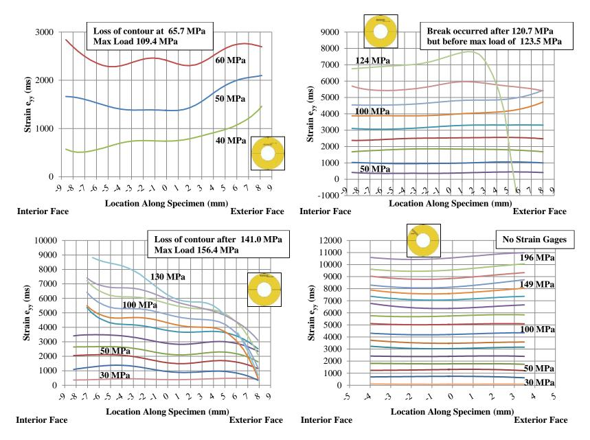
Figure A-16: Specimen TG1-11 (Fixed): Inner (Upper Left), Middle (Upper Right), Outer (Lower Left), & Radial (Lower Right)
