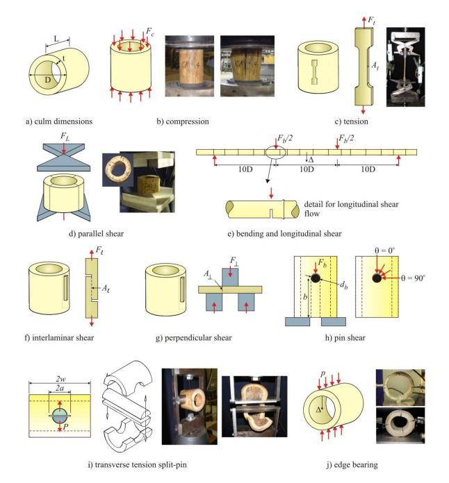
Figure 2-17: Current bamboo standards as well as proposed lab and field applicable tests (Harries et al. 2012)
