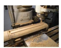
b) specimen fabrication in horizontal milling machineFigure 3-7: Tensile test specimens
