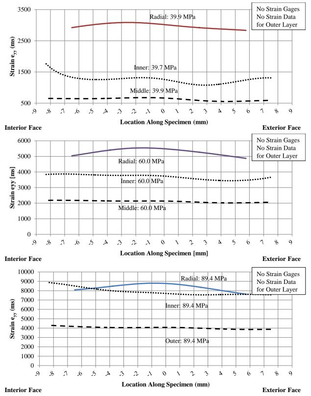
Figure 3-17: Strain profile for Specimen TG1-5 (fixed): 40MPa (top), 60MPa (center), and 89MPa (bot.)
