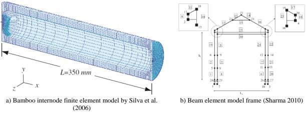
Figure 7-1: Modeling of structural bamboo components
