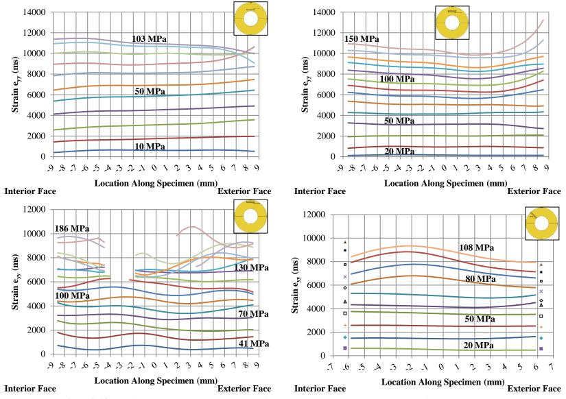
Figure 3-14: Specimen TG1-5 (Free): Inner (Upper Left), Middle (Upper Right), Outer (Lower Left), & Radial (Lower Right)
