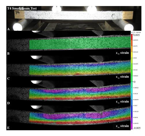
Figure 4-10: VIC-3D contour images for un-notched Tre Gai beam specimen
