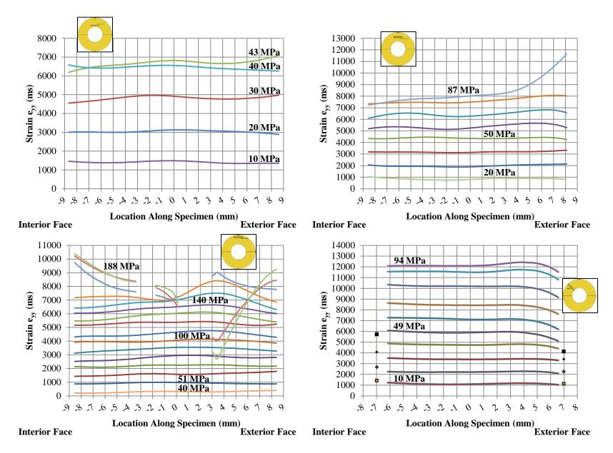
Figure A-17: Specimen TG21-11 (Free): Inner (Upper Left), Middle (Upper Right), Outer (Lower Left), & Radial (Lower Right)
