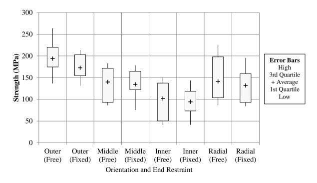
Figure 3-12: Experimental Tensile Strength
