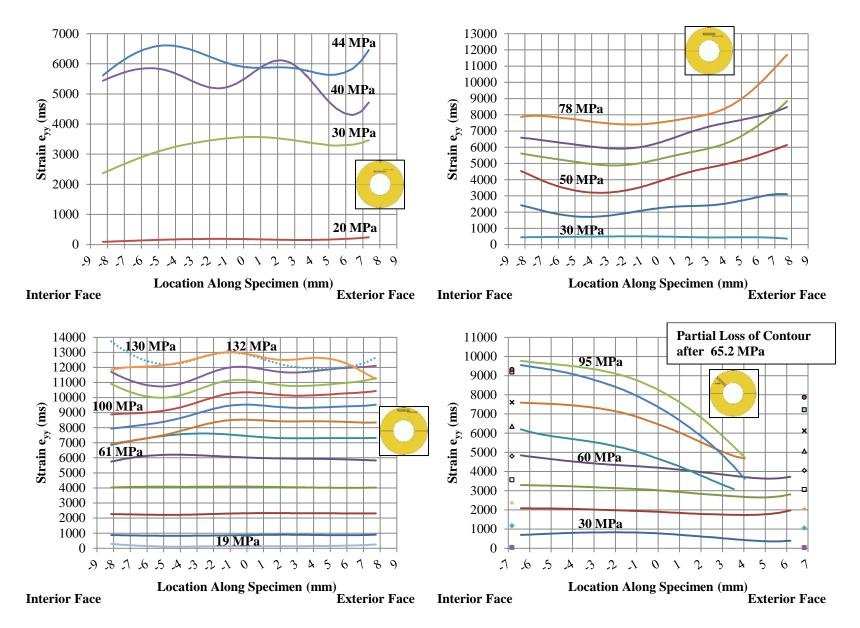
Figure A-18: Specimen TG21-11 (Fixed): Inner (Upper Left), Middle (Upper Right), Outer (Lower Left), & Radial (Lower Right)
