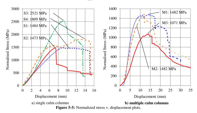
Because the tests are conducted in displacement control, critical buckling is identified as occurring at the load plateau in Figure 5-5 although lateral displacements of the culms is evident at lower loads. Eventual culm splitting (described below) corresponds to the subsequent, almost instantaneous, loss of capacity evident in the curves shown in Figure 5-5.
