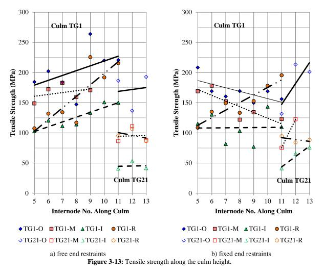
In summary, the tensile strength results illustrate the influence of machine-imposed end restraints and the location and orientation within the culm from which the tension specimen is extracted. The latter affects the fiber volume ratio in the test specimen. The mechanisms affecting these general trends in tension behavior are explored further in the following section in which strain patterns in the specimens are investigated.
