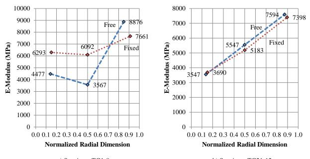
a) Specimen TG1-8 b) Specimen TG21-12 **Figure 3-19:** Representative E-Modulus profile for specimens TG1-8 and TG21-12
