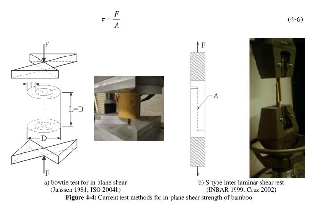
Cruz (2002) also developed a 'lap shear' test arrangement to study shear strength perpendicular to the longitudinal fibers. Sharma (2010) provides an extensive review of available bamboo test methods. Nonetheless, current available standardized tests do not investigate bamboo splitting characterized by the tensile strength perpendicular to the bamboo fibers (Mode I) or mixed-mode failures.
