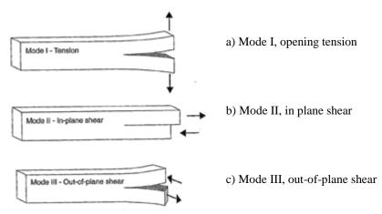
Figure 4-3: Standard definitions of fracture modes (Smith et al. 2003)
