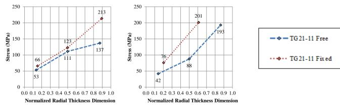
Figure A-46: Stress versus wall thickness location (cont.)
