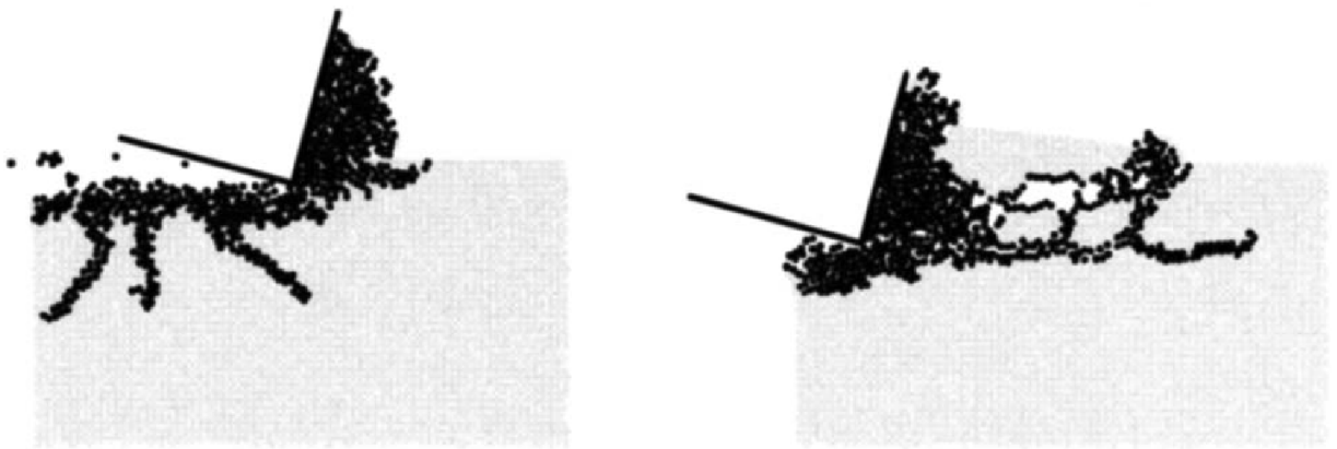
Figure 2.17 Ductile and brittle failure due to cutting depth and particle size ratio [26]
