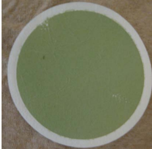
Figure 2.11 “Green deposits” retained on 0.45 \mu\text{m} filter paper after filtering the recirculating water in Tower B on day 9 in pilot scale tests with MWW_pH at pH 7.0
