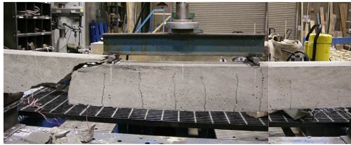
Figure 2.11 Photograph of beam C cracking after failure (collage of two images).
