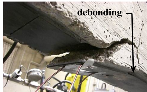
(b) Photograph of debonding failure.
