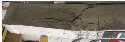
(b) Photograph of S-18-B cracking after failure.
