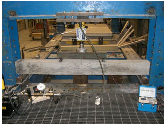
(b) Photograph of beam tests set-up.
