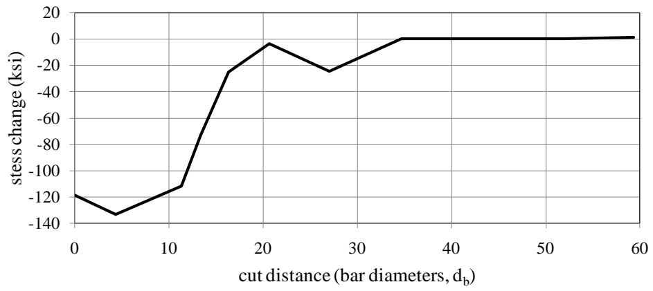
Figure 2-11 Stress drop versus cut distance.
