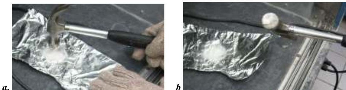
Figure 26. Falling hammer test of 88 : (a) appearance of 88 before striking with a hammer; (b) appearance of 88 after being struck with a hammer
